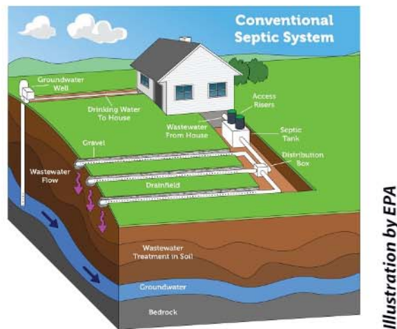
Figure 1: Typical composition of an on-site wastewater treatment system.
